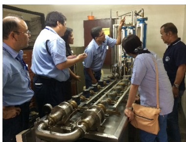
Water Meter Error Testing
